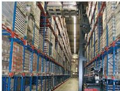
Double Deep Pallet Racking
