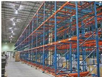
Push Back Pallet Racking
