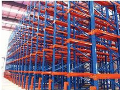
Drive-in Pallet Racking
